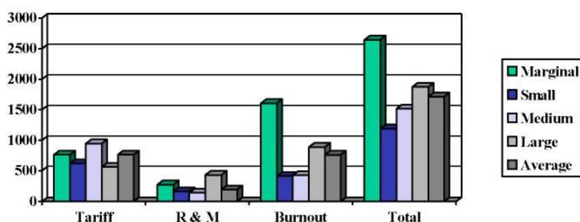
On a per hectare basis, the variable irrigation costs for electric pump owners was much higher for marginal farmers due to the regressive nature of the flat rate tariff structure and the cost of poor quality power (motor burnouts) Motor burnouts for marginal farmers cost, on per hectare basis, twice the electricity tariff cost.
